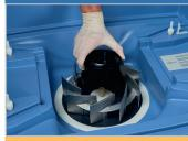
4 Insert fan impeller and connecting piece.
